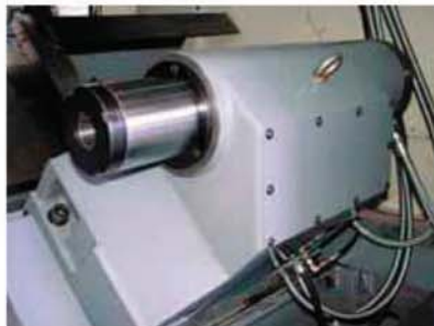
Tailstock for larger models with rotary quill.
