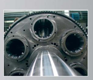
Spindle drum with locking rim
