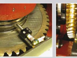
Detail of 4 independent overload release clutches
