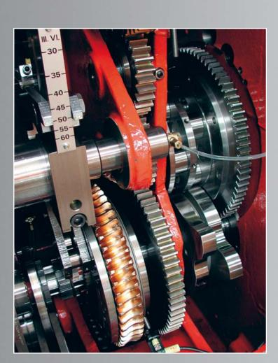
Spindle drum indexing mechanism with safety clutch
