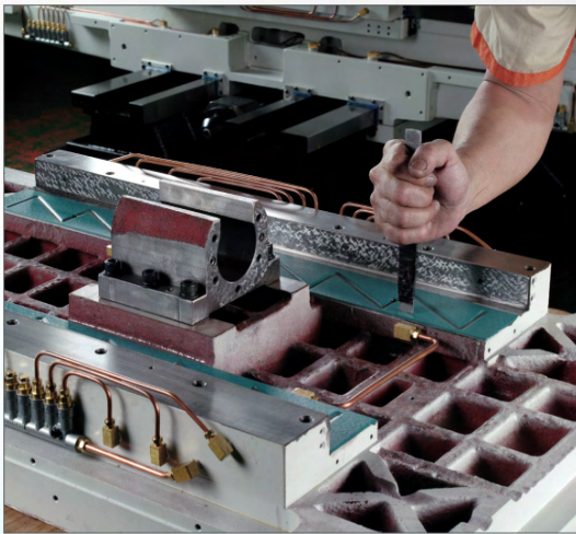
• Hand scraping All of the main assembling surfaces are hand scraped to optimize machine accuracy.
